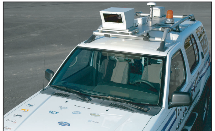
ILRIS-3D mounted on top of the “Xboxx” Nissan Xterra
